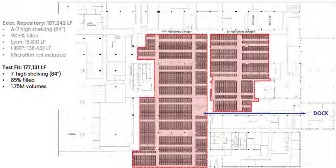
Figure 2.4 - 2550 Northwestern Avenue repository test fit for collections storage
